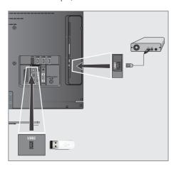
Connect the »USB1« socket of the television and the corresponding socket of the data medium (external hard disk) using a USB cable:
